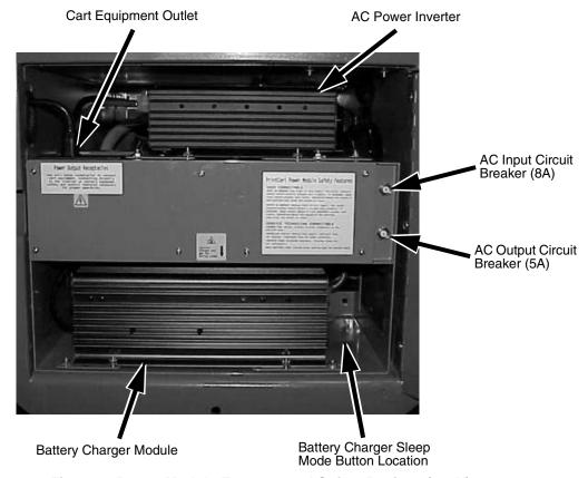
Figure 9. Power Module Features and Safety Devices (230V)
