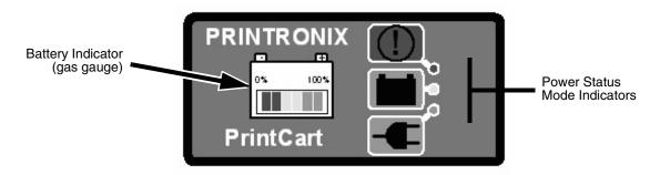
Figure 10. Display Panel Layout Indicator Colors
