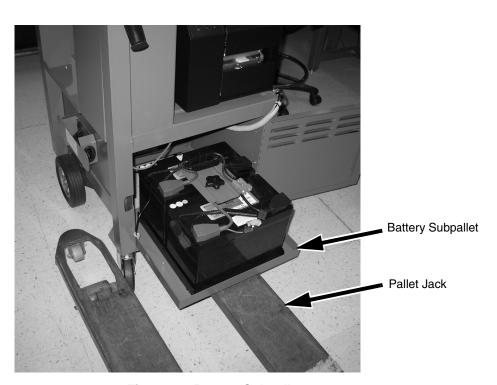
Figure 20. Battery Subpallet
