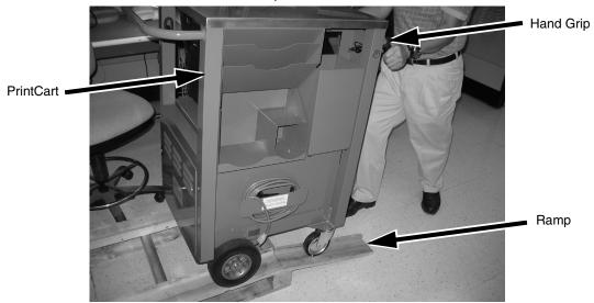
Figure 3. Moving the PrintCart to the Work Surface
