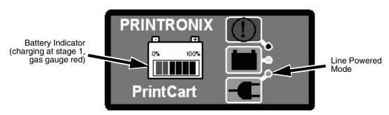
Figure 12. Operating in Unrestricted, Line Powered Mode
