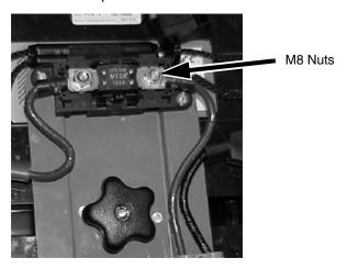
Figure 23. Replacing the Main DC Power Fuse
