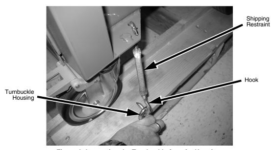
Figure 2. Loosening the Turnbuckle from its Housing
