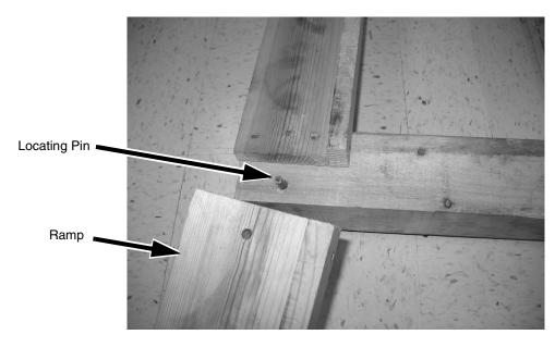
Figure 1. Reversing the Ramps and Engaging the Locating Pin
